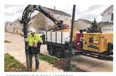
HYDRAULIC BOOM (OPTION). The hydraulic boom offers a 6-way function, wireless remote with vacuum valve operation, 330-degree rotation, remote water jet for ease of cleanout, and a 5-in (13-cm) hose with quick connect to 4-in (10-cm) tooling.
