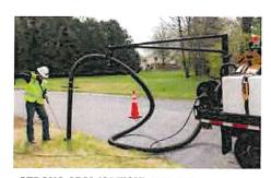
STRONG ARM (OPTION). With 270-degree rotation, the strong arm supports the weight of the vacuum hose, and the roller head makes handling efficient by allowing smooth, fluid movements and adjustments.
