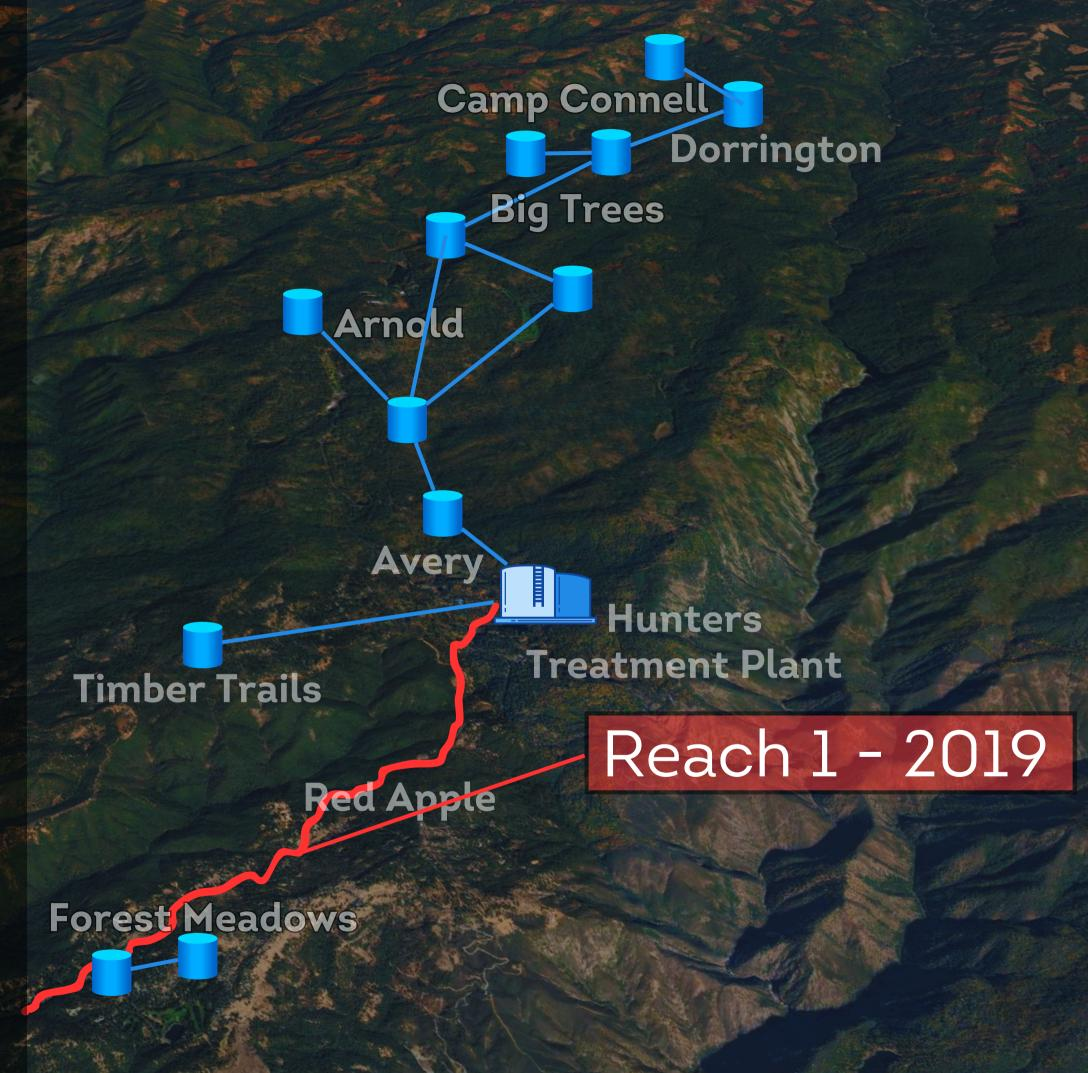
Replaced ten miles of Water Main with 10 & 12 inch Ductile Iron Pipe.
