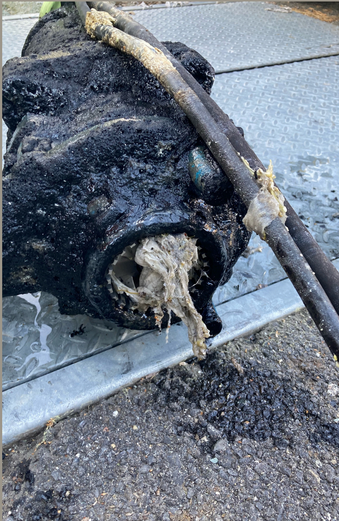
De-Ragged Pumps at Lift Station 10 - Poker Flat
