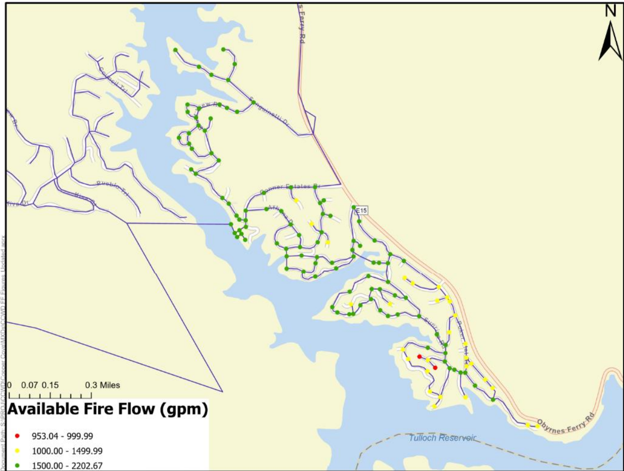
Figure 8. Alternative 2A - 12" Transmission Main
