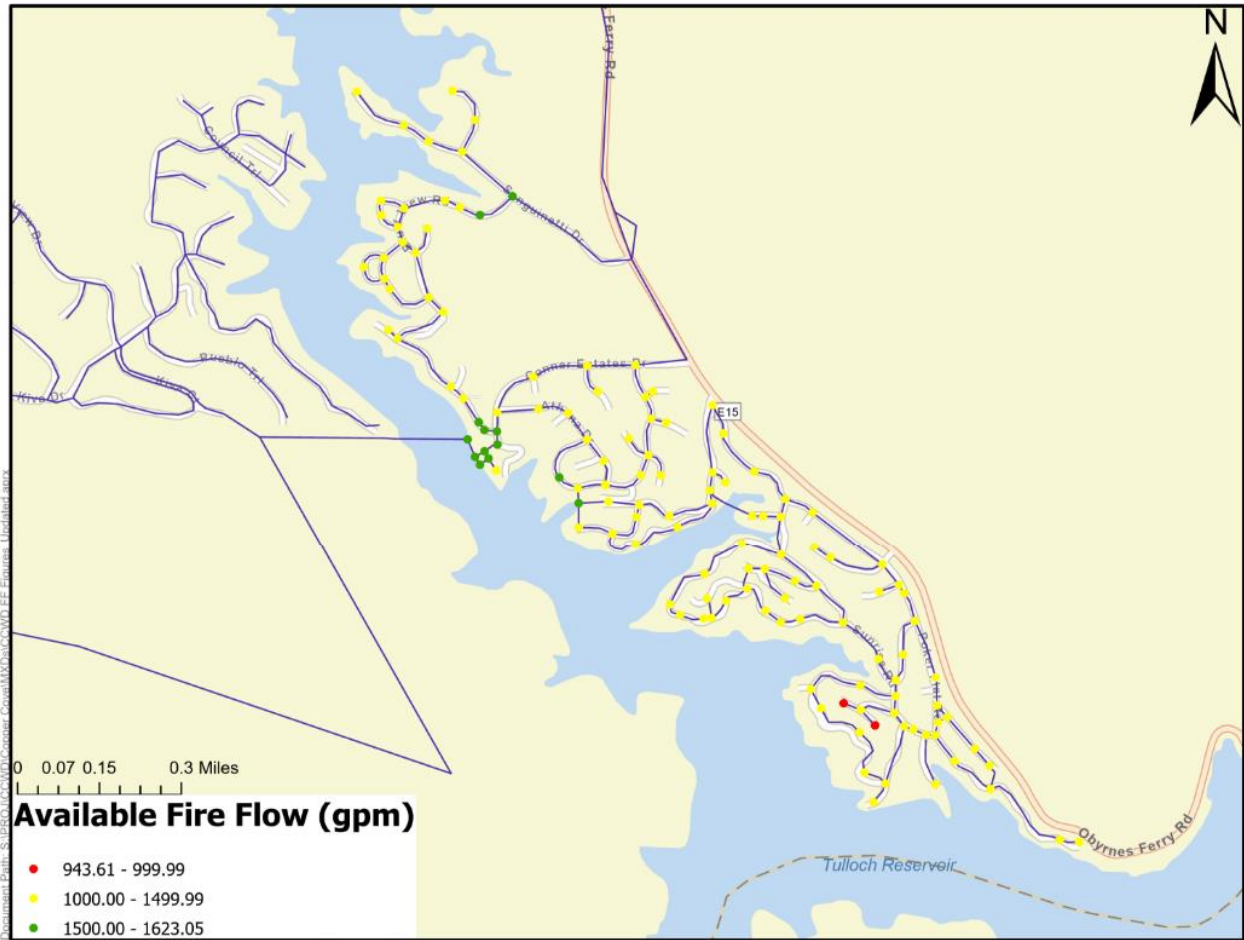
Figure 9. Alternative 2B - 10" Transmission Main
